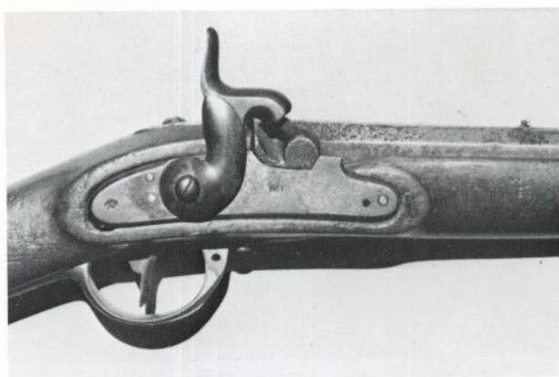
The Confederates imported some 27,000 0.54-calibre Austrian rifled muskets. The lockplate on this one is dated 1861. (Author's collection)
